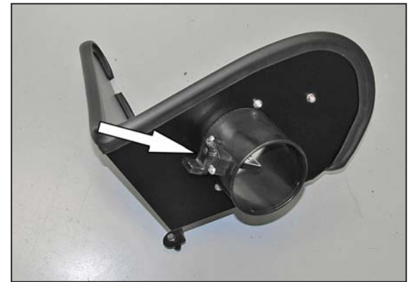
19. Install the mass air sensor into the K&N® mass air housing and secure with the provided hardware.
