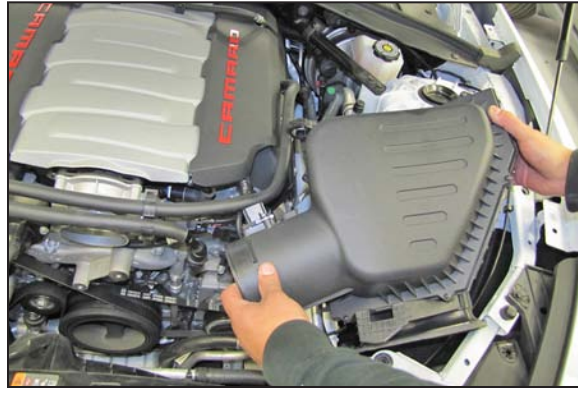
12. Lift up the air filter housing to dislodge it from the mounting grommets and then remove it from the vehicle.
