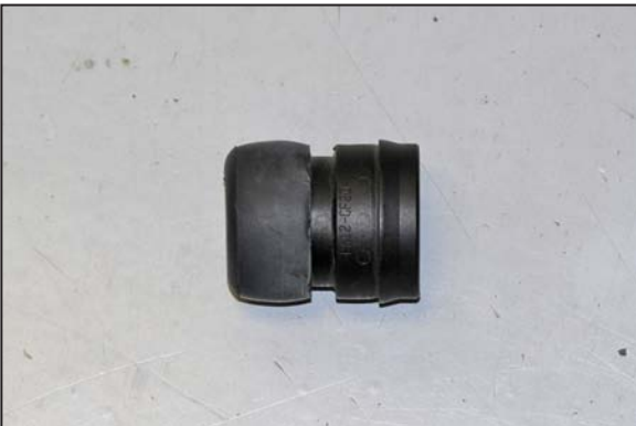
10. Install the provided cap onto the quick disconnect union.
