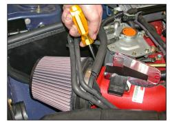
29. Install the K&N<sup>®</sup> air filter and and secure with the provided hose clamp as shown.
