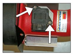
18. Install the mass air sensor from step 7 into the K&N<sup>®</sup> intake tube and secure with the provided hardware as shown.
