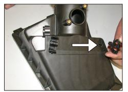
19. Remove one of the hose clips from the stock airbox assembly as shown.
