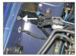
10. Remove the bolt on the wire harness bracket on the inner fender as shown.
