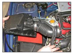
6. Remove the upper air cleaner assembly as shown.
