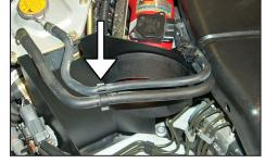
23. Reinstall the hose clip from step 22 and locate as shown.
