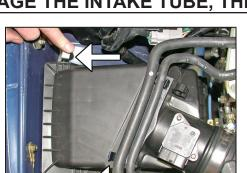
5. Unclip the upper air cleaner assembly as shown.
