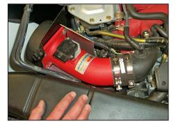
21. Install the complete assembly into the vehicle and slide the tube into the silicone hose as shown.
