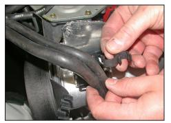
22. Remove the coolant hose clip as shown.
