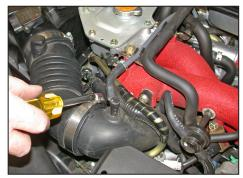
4. Loosen the hose clamp as shown.
