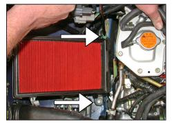
8. Remove the two bolts that secure the lower air cleaner assembly as shown.
