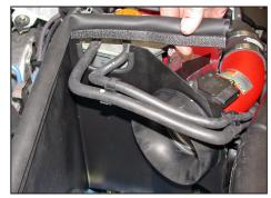
28. Install the remaining trim seal onto the heat shield and trim to fit as shown. **NOTE: Some trimming of the edge trim may be**
