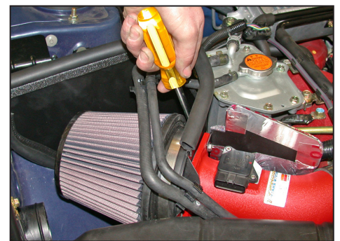
29. Install the K&N® air filter and secure with the provided hose clamp as shown.
