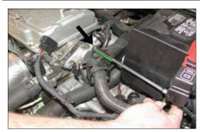
10. Remove the bolt that secures the wire harness to the engine as shown.
