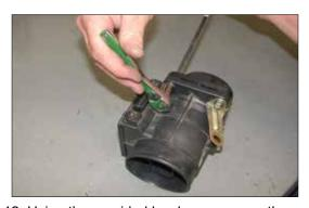
12. Using the provided hardware, secure the provided mass air adapter and the wire harness bracket to the stock mass air sensor as shown.
