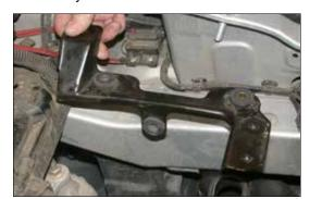
8. Loosen and remove the two bolts that secure the air cleaner support bracket, then, remove the air cleaner support bracket as shown.
