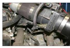
21. Re-clip the mass air sensor wire harness to the stock bracket on the mass air sensor as shown.
