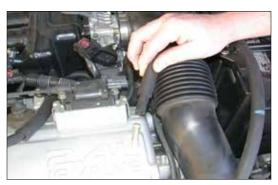
3. Disconnect the crank case vent hose from the cam cover as shown.
