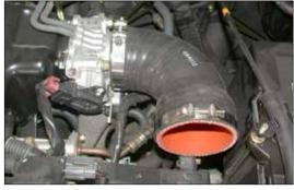
14. Install the 90 degree silicone hose onto the throttle body as shown.
