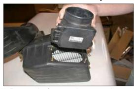
11. Remove the four nuts that secure the mass air sensor, then, remove the mass air sensor as shown.
