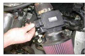
20. Reconnect the mass air sensor electrical connection as shown.
