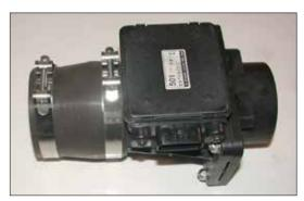
13. Install the silicone step hose and hose clamps onto the mass air sensor as shown.
