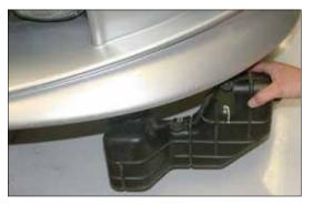
9. From underneath the vehicle remove the lower valance and loosen the three bolts that secure the air intake resonator to the inner fender, then, remove the air intake resonator from underneath the vehicle as shown.
