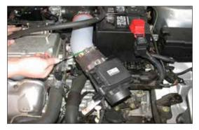
17. Slide the mass air sensor assembly onto the Typhoon intake tube as shown.
