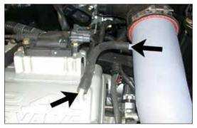
18. Install the provided silicone hose onto the vent on the cam cover, then, slide the other end onto the vent on the intake tube as shown.
