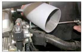
16. Using the provided hardware secure the tube bracket to the threaded boss from step 8 as shown.
