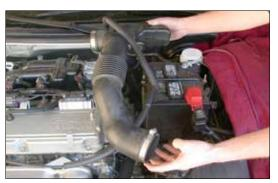
4. Loosen the hose clamps at the throttle body and at the mass air sensor, then, remove the stock intake tube as shown.
