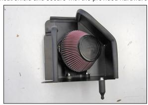
15. Install the K&N<sup>®</sup> air filter onto the filter adapter and secure with the provided hose clamp.
