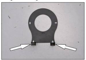
9. Install the two male/female rubber mounted studs onto the filter mounting bracket using the provided hardware.
