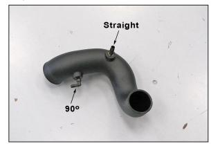
21. Install the 90° and straight vent fitting into the  $K\&N^{\otimes}$  intake tube as shown.
