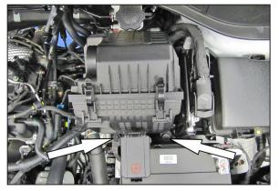
8. Remove the two bolts that secure the air filter housing and then remove the air filter housing from the vehicle.
