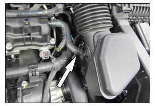
4. Release the spring clamp securing the crank case vent hose to the intake tube and then disconnect the crank case vent hose from the intake tube.
