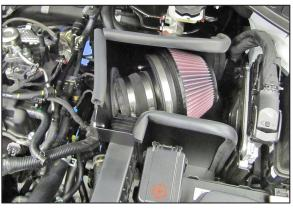
20. Install the provided step coupler (08496) onto the filter adapter and secure with the provided hose clamp.
