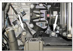
17. Install the heat shield assembly onto the rubber mounted studs and insert the mounting post into the mounting grommet. Secure the heat shield with the hardware provided.
