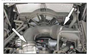
5. Loosen the two hose clamps that secure the factory intake tube to the throttle body and to the air filter housing and then remove the factory intake tube from the vehicle.
