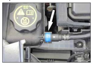
10. WARNING: Be sure the engine is completely cool before proceeding with this step! Release the blue locking tap securing the factory coolant hose to the expansion tank and then disconnect the hose from the tank.
