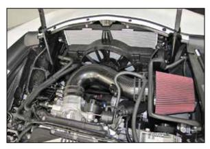
24. Install the K&N® intake tube into the heat shield and air filter and then into coupling hose at the throttle body. Adjust the tube and filter for best fit and then secure with the provided hose clamps.
