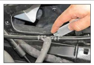
11. Using a razor knife, cut the plastic hose at the TEE fitting as shown. Separate the hose from the TEE fitting.
