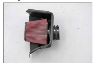
18. Set the air filter into the heat shield and then install the coupling hose (08761) onto the filter and secure with the provided hose clamp.
