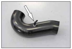
23. Install the provided 90° npt fitting into the K&N $^{\circ}$  intake tube as shown.
