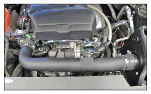
28. Install the K&N<sup>®</sup> intake tube assembly onto the filter adapter and then onto the throttle body. Adjust the tube and step hose for best fit and then secure with the provided hose clamps.
