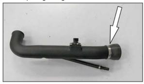
26. Install the provided Step coupler onto the K&N<sup>®</sup> intake tube as shown.
