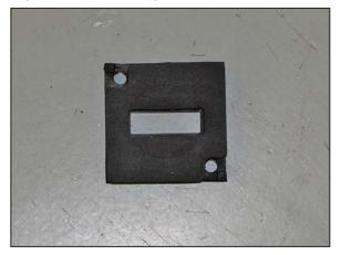
22. Install the provided gasket onto the K&N<sup>®</sup> mass air adapter.
