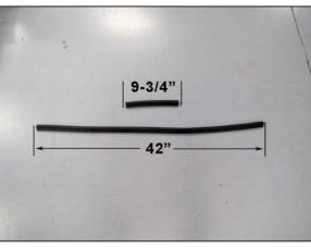
14. Cut the provided edge trim into two sections as shown. One section is 9-3/4" long and the other section is 42"long.
