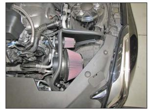
18. Install the heat shield assembly into the engine compartment so the mounting studs go into the mounting grommets and the insert nut goes into the front mounting grommet location. Secure the heat shield by tightening the bolt into the insert nut.
