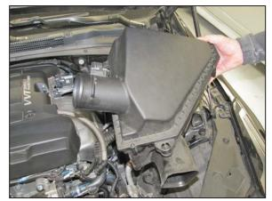
8. Lift up the air filter housing to dislodge it from the mounting grommets and then remove it from the vehicle.
