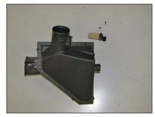
23. Remove the mass air sensor from the air filter housing.
