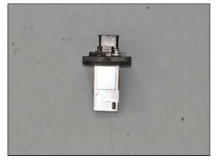
24. Install the mass air sensor into the K&N<sup>®</sup> adapter and secure with the provided hardware.
