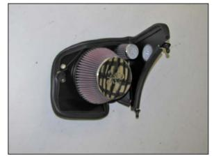
17. Install the K&N $^{\odot}$  air filter onto the filter adapter and secure with the provided hose clamp.
