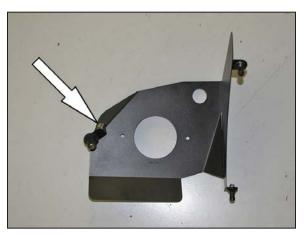
12. Install the bracket assembly onto the heat shield but do not completely tighten at this time.
