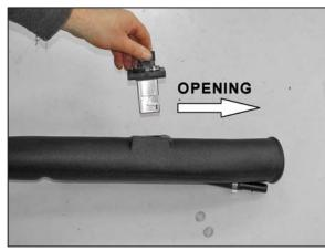
25. Install the mass air sensor into the K&N<sup>®</sup> tube with the opening facing the direction shown.
