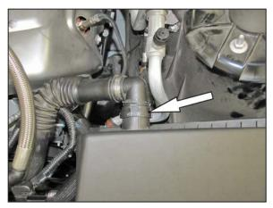
7. Disconnect the secondary air hose from the air filter housing.
