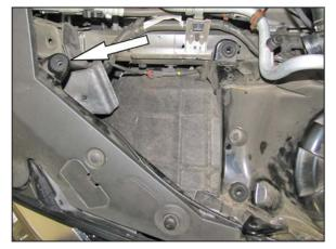
9. Remove the forward most air filter housing mounting grommet shown.
