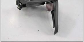
16. Install the secondary air filter onto the heat shield using the provided adapter. NOTE: On vehicles that are not equipped with a secondary air system it is not necessary to install the breather filter. 21. Install the vent hose assembly onto the fitting installed into the  $K\&N^{\otimes}$  intake tube and secure with the provided hose clamp.
