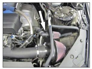
30. On vehicles equipped with secondary air, connect the secondary air hose to the adapter installed into the Heat shield as shown. NOTE: It will be necessary to twist the 90° fitting in the hose so that it will connect with the adapter.
