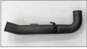
19. Install the provided vent fitting into the K&N<sup>®</sup> intake tube.
