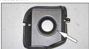
11. Install the filter adapter into the heat shield and secure with the provided hardware.
