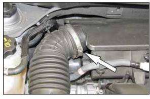
4. Loosen the hose clamp that secures the intake tube to the intake plenum.
