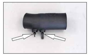
6. Install the two provided vent fittings into the K&N^ $^{\odot}$  intake tube as shown.
