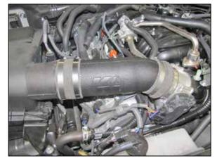
9. Install the K&N<sup>®</sup> intake tube assembly into the coupling hoses, secure the air box lid with the factory retaining clips and then secure the tube with the provided hose clamps.
