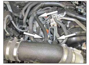
11. Install the crank case vent hose assembly into the factory crank case vent hose and then connect the open end to the fitting installed into the K&N<sup>®</sup> intake tube. Connect the factory fuel pressure regulator vent hose into the fitting installed into the K&N<sup>®</sup> intake tube.
