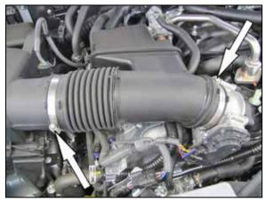
4. Loosen the two hose clamps securing the factory intake tube to the throttle body and air filter housing and then remove the factory intake tube. **NOTE: K&N Engineering, Inc., recommends that**
