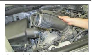
5. Remove the factory intake tube from the vehicle. NOTE: K&N Engineering, Inc., recommends that customers do not discard factory air intake.
