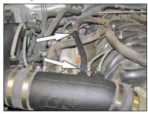
13. Install the union fitting into the K&N® crank case breather hose and then connect the hose to the factory crank case vent hose and the fitting installed into the K&N® intake tube.
