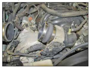
9. Install the provided hump coupling hose (08699) onto the throttle body and secure with the provided hose clamp.
