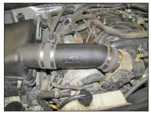
11. Lift up the upper air filter housing, install the K&N® intake tube into the silicone hoses and then reinstall and latch the upper air filter housing. Adjust the tube for best fit and then secure with the provided hose clamps.
