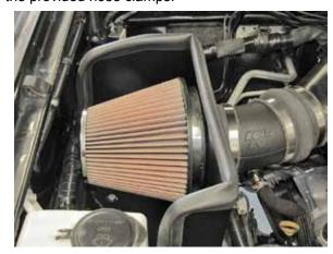
28. Install the K&N® air filter onto the filter adapter and secure with the provided hose clamp.
