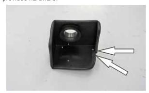
19. Install the provided edge trim around the perimeter of the heat shield as shown.
