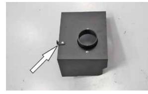
17. On 2012 and later model year vehicles, install the heat shield mounting bracket (064318) onto the heat shield as shown using the provided hardware.
