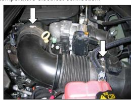
3. Loosen the hose clamps that secure the factory intake tube to the turbo inlet and air box.
