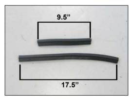
8. Cut the provided edge trim into two sections as shown, one is to be 9.5" long and the other section is to be 17.5" long.
