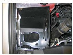
11. Set the heat shield into position on the air box tray and then secure to the air box tray using the provided hardware.
