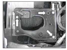
7. Remove the air box mounting grommet and mounting plate bolts shown.
