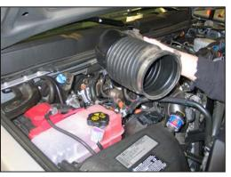
4. Remove the factory intake tube from the vehicle.
