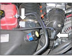
2. Disconnect the mass air sensor and the temperature electrical connection.
