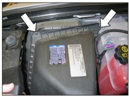
5. Loosen the two screws securing the air box lid and then remove the air box lid and air filter.
