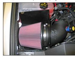
15. Install the K&N® intake tube into the heat shield and secure with the provided hardware. Then install the K&N® air filter onto the intake tube and secure with the provided hose clamp.
