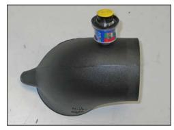
14. On vehicles that are equipped with a filter minder, install the provided grommet and the factory filter minder into the K&N® intake tube as shown. On vehicles not equipped with a filter minder, Install the provided plug.
