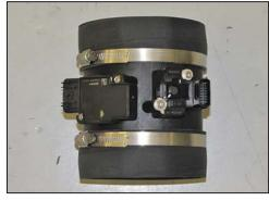
18. Install the two provided silicone hoses (08495) onto the K&N<sup>®</sup> mass air sensor housing as shown; secure with the provided hose clamps.
