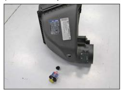
13. Remove the filter minder and grommet from the factory air box.
