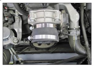
8. Install one of the provided coupling hoses onto the throttle body and secure with the provided hose clamps.
