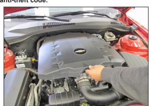
2. Remove the oil fill cap and then lift up the engine cover and remove it from the engine. Reinstall the oil fill cap at this time.
