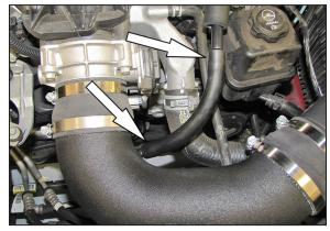
12. Connect the provided crank case breather hose onto the fitting installed into the K&N® intake tube and then attach the open end to the factory crank case vent tube.
