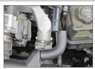
3. Disconnect the Crank case vent hose from the crank case vent tube.
