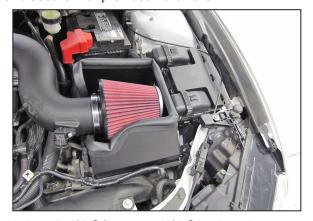
18. Install K&N® filter onto K&N® intake tube. Secure with provided hose clamp.
