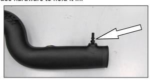
14. Install provided  $1\!\!/_{\!\!4}$  NPT quick connect fitting onto the K&N® intake tube.
