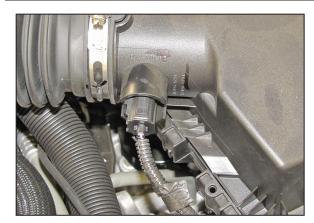
6a. Some vehicles may be equipped with a twist lock style temperature sensor.
