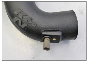
13. Install the temperature sensor into the K&N® intake tube and secure with the provided hardware. NOTE: The quarter turn style sensor does not use hardware to hold it in.
