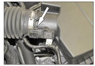
6. Disconnect the temperature sensor electrical connect.
