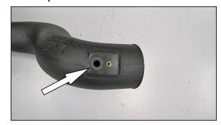
12. Install provided grommet into K&N® intake tube
