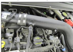
19. Connect crankcase vent line onto quick connect fitting on K&N® intake tube.
