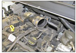
9. Install the coupling hose (08690) onto factory turbo intake tube and secure with provided hose clamp.
