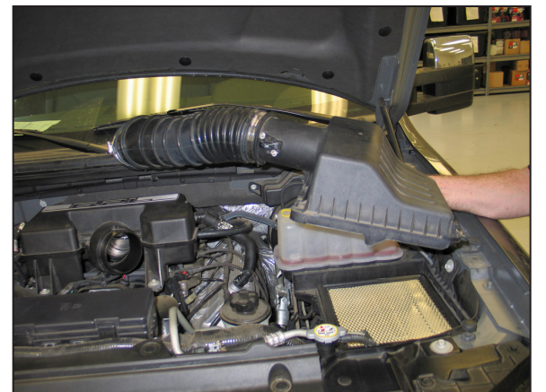
5. Remove the upper air box/intake hose assembly and air filter.
