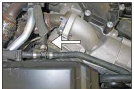
2. Release the red locking tab and then disconnect the mass air sensor electrical connection and unhook the wiring harness from the air box.
