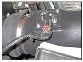
35. Reconnect the mass air sensor electrical connection. Secure the mass air sensor wiring harness to the A/C recharge pipe with the provided tie wrap.
