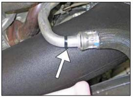
32. Secure the coolant pipe to the insert of the  $K\&N^{\textcircled{o}}$  intake tube with the provided mounting tie wrap.
