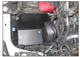
14. Unhook the wiring harness from the fresh air intake duct.
