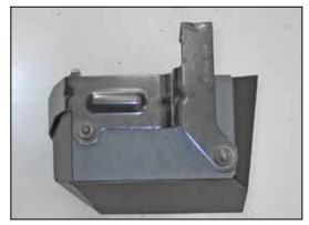
22. Install the factory air box mounting bracket onto the heat shield as shown so that the mount stand-offs installed in step #20 snap into the factory mounting grommets.
