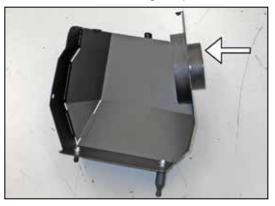
21. Install the filter adapter into the heat shield using the provided hardware.
