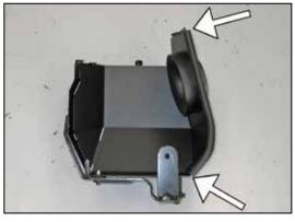
23. Install the provided edge trim onto the heat shield as shown.
