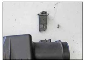
27. Remove the two screws securing the mass air sensor into the factory air box and then remove the sensor from the air box.
