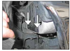
16. Remove the two clips shown that retain the bottom of the fresh air intake duct.
