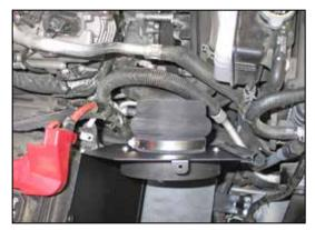
25. Install the silicone hump hose (08418) onto the filter adapter and secure with the provided hose clamp.
