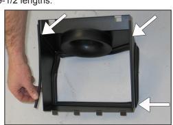
12. Install the two 9-1/2" lengths of small edge trim onto the bottom heat shield as shown.
