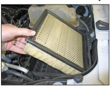
7. Remove the air filter from the lower air box.
