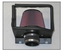
14. Install the provided silicone hose (08699) onto the filter adapter as shown and secure with the provided hose clamp.
