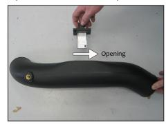
20. Install the mass air sensor assembly into the K&N® intake tube as shown.
