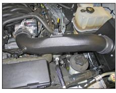
22. Install the K&N® intake tube; insert the lower end into the silicone hose attached to the heat shield /air filter assembly. Attach the upper end of the intake tube to the silicone hose secured to the throttle body. Secure the intake tube with the provided hose clamps.
