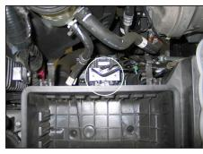
8. Remove the center upper air box retaining clip from the lower air box.
