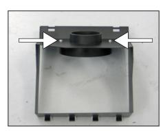
9. Install the K&N $^{\odot}$  filter adapter into the heat shield as shown and secure with the provided hardware.
