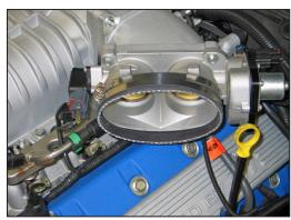
19. Install the provided silicone hose (08627) onto the throttle body and secure with the provided hose clamp.
