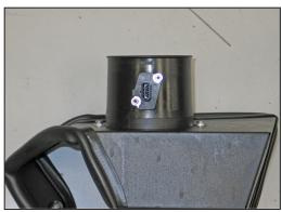
13. Install the mass air sensor into the K&N® mass air sensor housing and secure with provided hardware.
