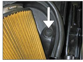
3. Remove the bolt that secures the airbox housing to the inner fender.
