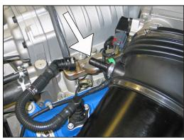
5. Rotate the locking ring and then disconnect the crankcase vent hose as shown.
