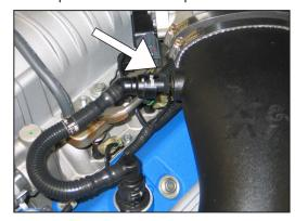
22. Connect the crankcase vent line to the quick disconnect fitting installed into the K&N® intake tube.
