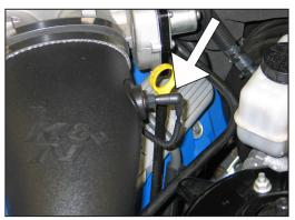
23. Connect the vent line to the 3/16" fitting installed into the K&N® intake tube.
