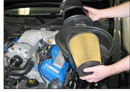
7. Disconnect the intake tube from the throttle body and then remove the complete intake system from the vehicle.
