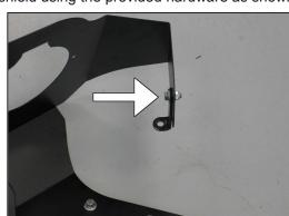
9. Install the heat shield mounting bracket (07158) onto the heat shield using the provided hardware.
