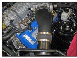
21. Install the K&N® intake tube into the silicone hose at the throttle body and align with the mass air sensor housing. Slide the silicone hose down the K&N® intake tube onto the mass air sensor housing. Align the tube for best fit and then secure with the provided hose clamps.
