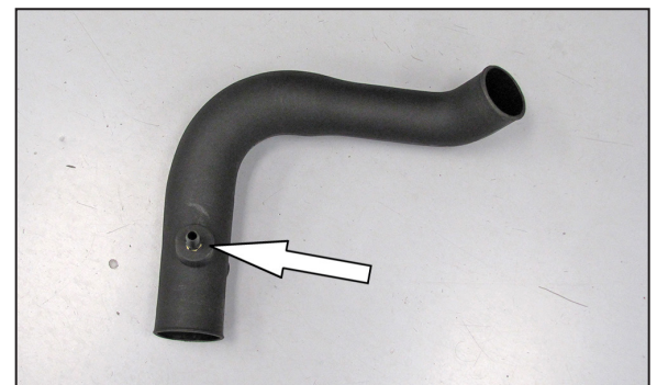
19. Install the provided vent fitting into the K&N® intake tube as shown.
