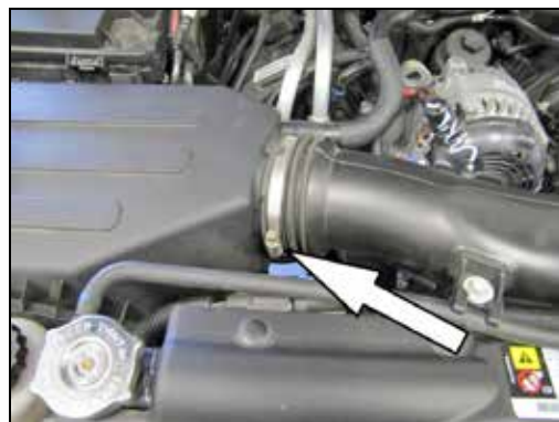
4. Loosen the hose clamp securing the factory intake tube to the air filter housing.
