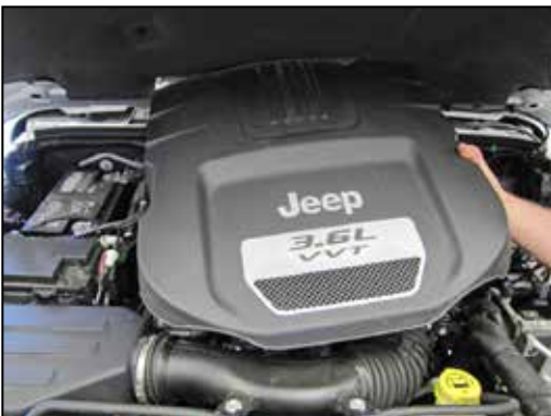
2. Lift up and remove the engine cover.
