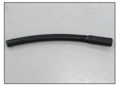
20. Assemble the two vent lines together using the provided hose mender.
