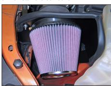
24. Install the  $K\&N^{\odot}$  air filter and secure with the provided hose clamp.
