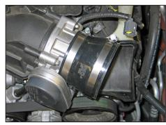
14. Install the silicone step hose (08497) onto the throttle body and secure with the provided hose clamp.
