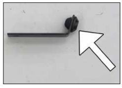
20. Install the mounting grommet from the intake plenum into the provided tube bracket as shown.
