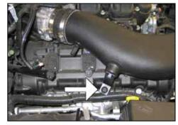
21. Install the K&N<sup>®</sup> intake tube into the silicone hump hose and then into the throttle body silicone hose. Install the tube bracket onto the mounting stud and secure it to the K&N<sup>®</sup> intake tube with the provided hardware. Tighten the hose clamps at this time.
