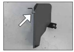
9. Install the heat shield mounting bracket (070066) onto the heat shield as shown using the provided hardware and spacer.
