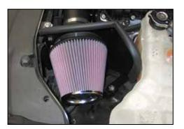
24. Install the K&N<sup>®</sup> air filter and secure with the provided hose clamp.
