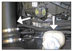
23. Install the provided silicone hose onto the factory crank case vent tube and then connect the open end to the 90° fitting installed into the K&N<sup>®</sup> intake tube.
