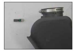
16. Rotate the inlet air temperature sensor counter clockwise and then remove from the factory intake tube.
