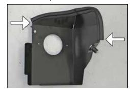
10. Install the provided longer edge trim onto the top of the heat shield as shown. NOTE: trimming of the edge trim will be necessary.
