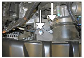
3. Remove the intake plenum mounting bolt shown and loosen the intake tube hose clamp.
