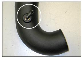
21. Install the 90° npt fitting into the K&N $^{\mbox{\tiny B}}$  intake tube as shown.
