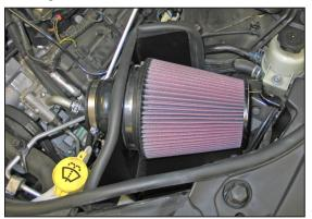
16. Install the K&N<sup>®</sup> filter onto the adapter and secure with the provided hose clamp. NOTE: Drycharger<sup>®</sup> air filter wrap; part # RF-1041DK is available to purchase separately.
