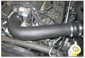
22. Install the K&N<sup>®</sup> intake tube into the silicone hump hose and then into the silicone hose at the throttle body, secure the intake tube with the provided hose clamp.
