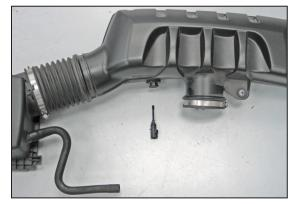
18. Release the locking tab and the remove the inlet air temperature sensor from the factory intake tube by twisting counter clockwise.
