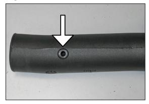
19. Install the provided grommet into the K&N $^{\mbox{\ensuremath{\$}}}$  intake tube as shown.
