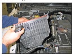
6. Lift up the lower air box to dislodge it from the mounting grommets and then remove it from the vehicle.
