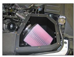
20. Set the K&N® air filter into the K&N® air box as shown.
