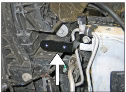
8. Install the air box mounting bracket (083145) onto the core support using the bolt removed in the previous step.
