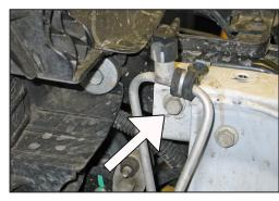
7. Remove the core support bolt shown. **NOTE: This bolt will be reused in the next step.**
