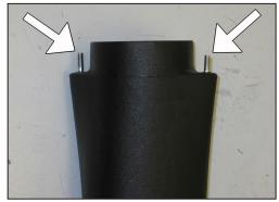
14. Install the two remaining 6mm studs into the fresh air intake scoop so the shorter threads are threaded into the inserts as shown.
