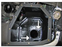
16. Secure the top of the fresh air intake scoop to the airbox with the provided hardware.
