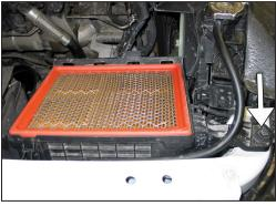
5. Remove the bolt that secures the lower air box to the core support.
