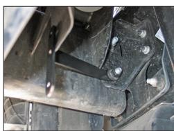
13. Install the tube mounting bracket (083157) onto the stud as shown and secure with the factory nut removed in the previous step.
