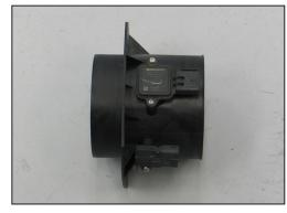
18. Install the mass air sensor and temperature sensor into the K&N® mass air sensor housing using a twisting motion to aid installation; secure with the provided hardware.
