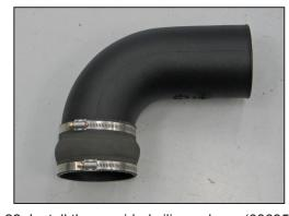
22. Install the provided silicone hose (08695) and hose clamps onto the K&N $^{\odot}$  intake tube as shown. NOTE: Do not completely tighten at this time.
