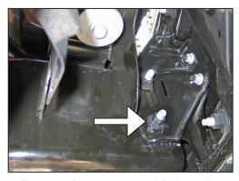
12. Remove the passenger side lower bumper mounting bracket nut shown.
