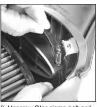
6. Unscrew filter clamp bolt and leave clamp undone. Place loosened clamp inside air box around flange base while installing K&N filter.
