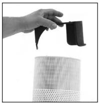
3. Remove the dirty air filter and remove the screw that fastens the top plate to the filter and depress the four tabs to release the top plate from the filter.
