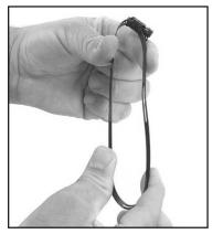
5. Squeeze the clamp supplied with the K&N filter as shown to conform to the filter base flange.
