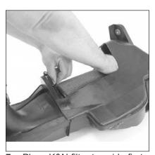
7. Place K&N filter top side first into air box. Position filter so that it can be pulled toward air box flange. Use pull tabs built into filter base to assist pulling filter flange onto air box flange until filter is seated.
