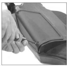
10. Install air filter cover and fasten screws.
