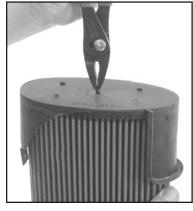
4. Install the top plate from the old filter onto the K&N filter. Using a pair of pliers, pull the rubber tip from the K&N filter through the hole on the filter top plate.
