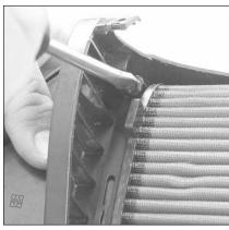
9. Position clamp over K&N filter flange and tighten.
