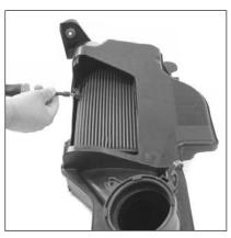
8. Once K&N filter is slid onto air box flange, install screw that retains filter in place.
