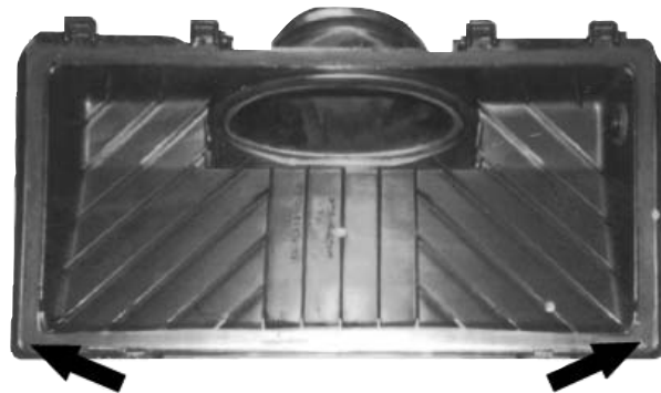
Apply gasket around edge of airbox.
