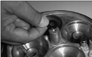
2) Apply spacer onto carburetor center post.
