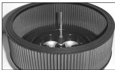
8) Place the K&N filter charger onto the base plate making sure it is fully seated.
