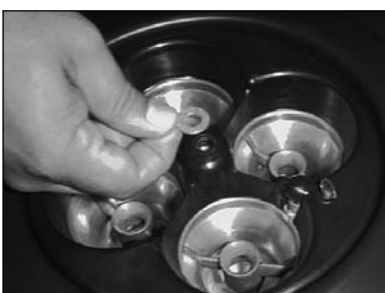
5) Place the small flat metal washer onto the K&N Stub Stack.
