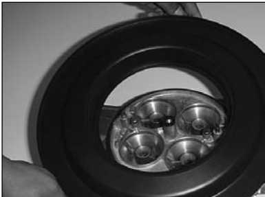
3) Place K&N base plate onto carburetor.
