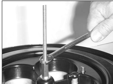
7) Screw the provided all-thread stud into stud adapter until it bottoms out. Secure it with the jam nut.
