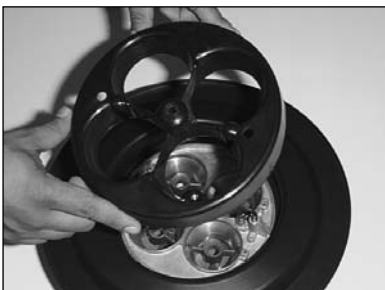
4) Place the K&N Flow Control Stub Stack onto base plate. NOTE: make sure the spacer remains in place when placing the stub stack onto the carb post.
