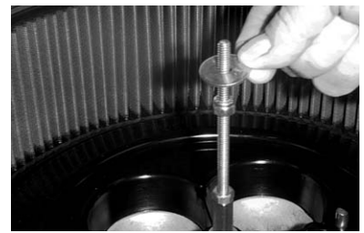
12) Install the provided flat washer.
