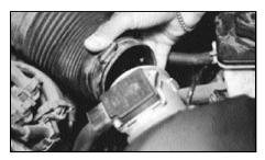
Loosen the mass <u>air intake tube</u>
