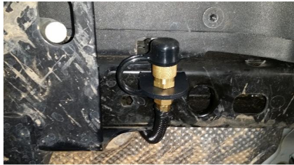
Figure 20 – Example of Air Coupler Mounted To Bumper
