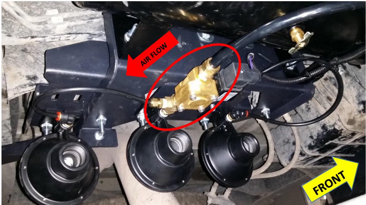
Figure 22 – Air Horn Drivers and Solenoid Mounted with Air Tubing Connected (730 Shown)
