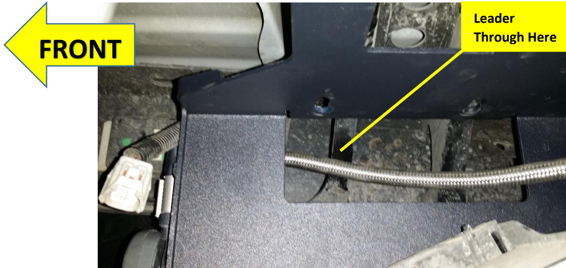
Figure 10 - Compressor Leader Hose Routing
