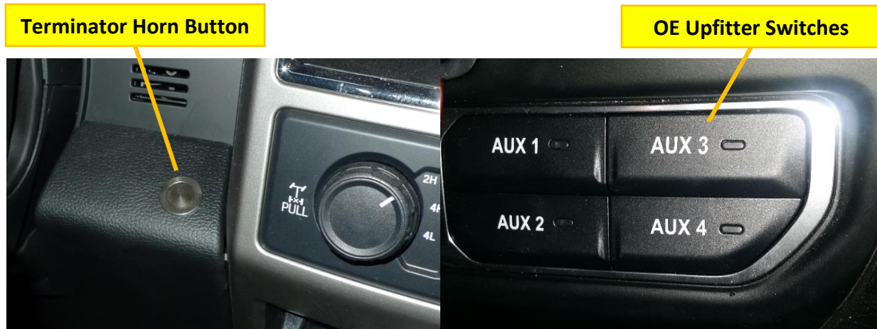
Figure 23 – Horn Button Installed in Dash (Shown in example vehicle)
