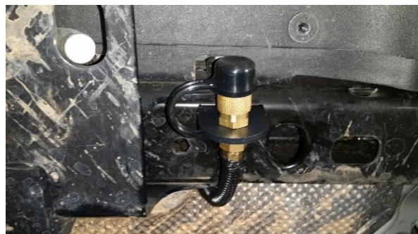
Figure 19 – Example of Air Coupler Mounted to Bumper
