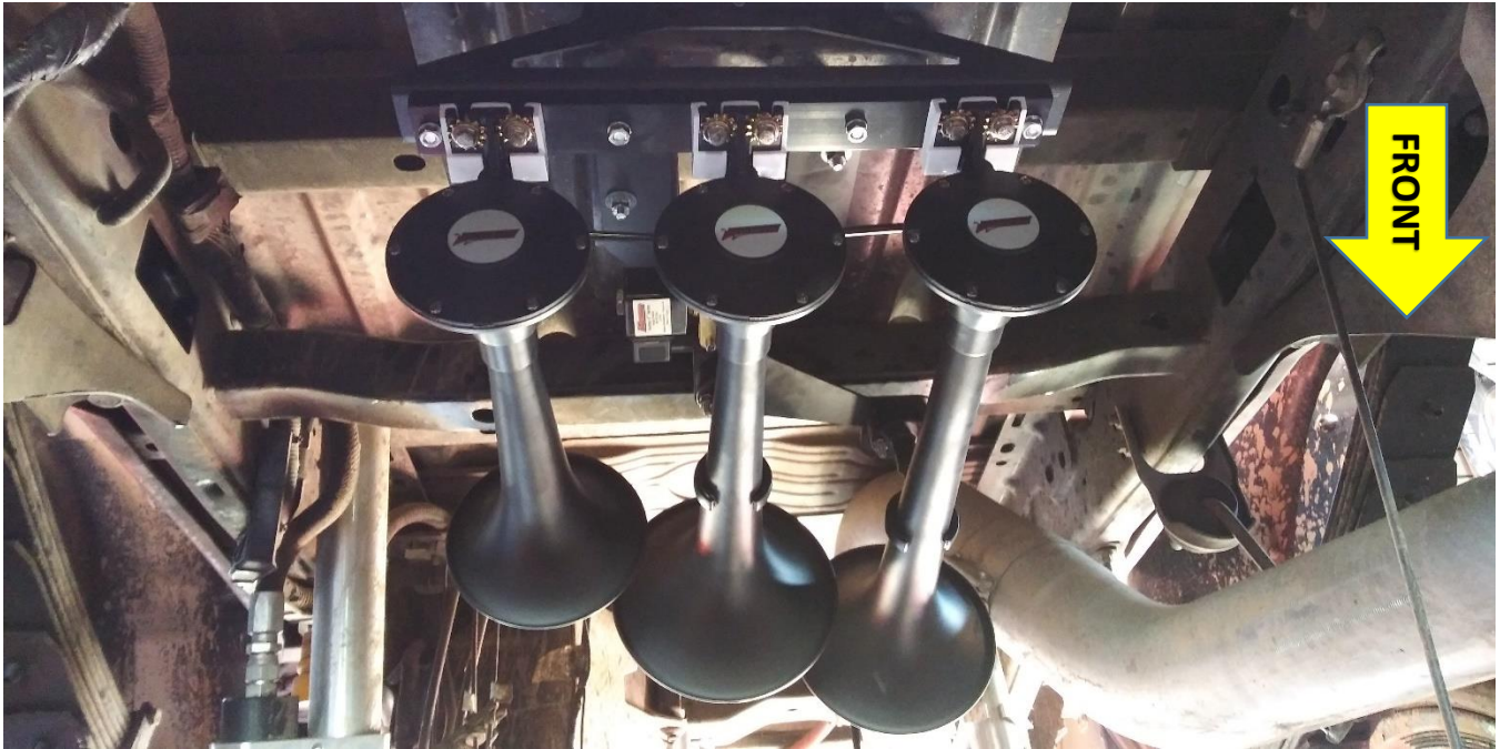
Figure 2 – Under Vehicle View of Air Horn Installed – without Air Tank & Compressor (2017 F-250 Shown)
