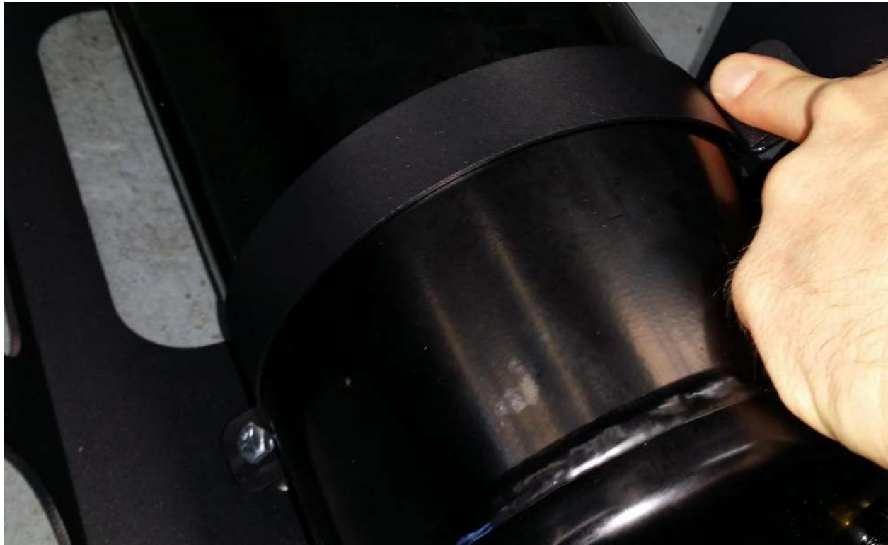
Figure 16 JK-202 Bent around Air Tank
