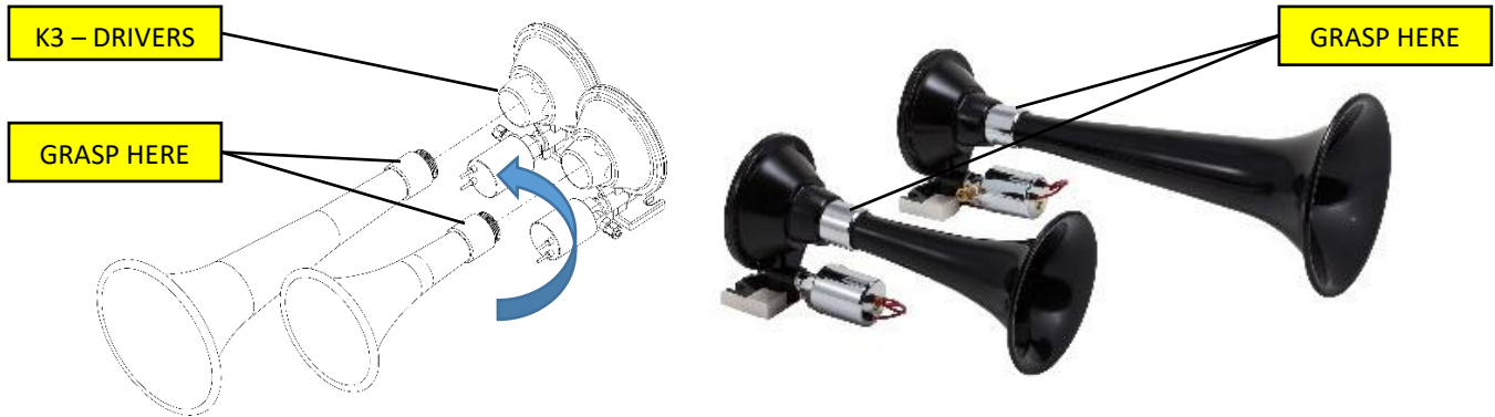
Figure 9 – Removing Trumpets from Air Horn Drivers, Exploded View
