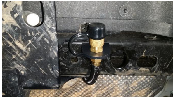
Figure 37 – Example of Air Coupler Mounted to Bumper
