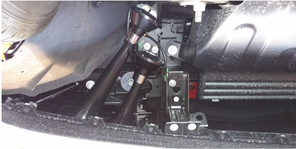
Figure 2 – Under Vehicle View of Air Horn Installed – Behind Front Bumper (2020 Silverado Shown)
