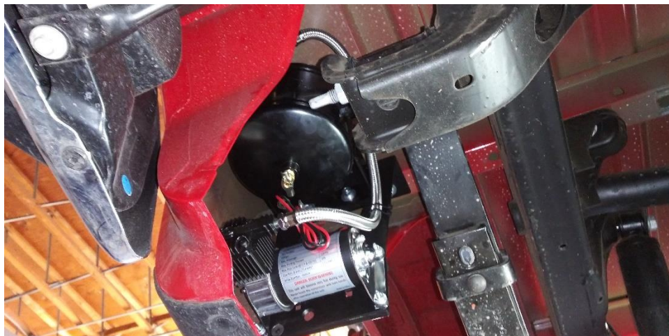
Figure 4 – Under Vehicle view of Air Compressor Installed – Behind Driver Wheel (2020 Silverado Shown)
