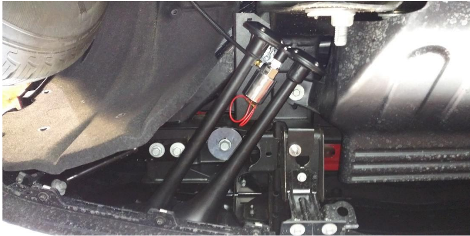
Figure 2 – Under Vehicle View of Air Horn Installed – Behind Front Bumper (2020 Silverado Shown)
