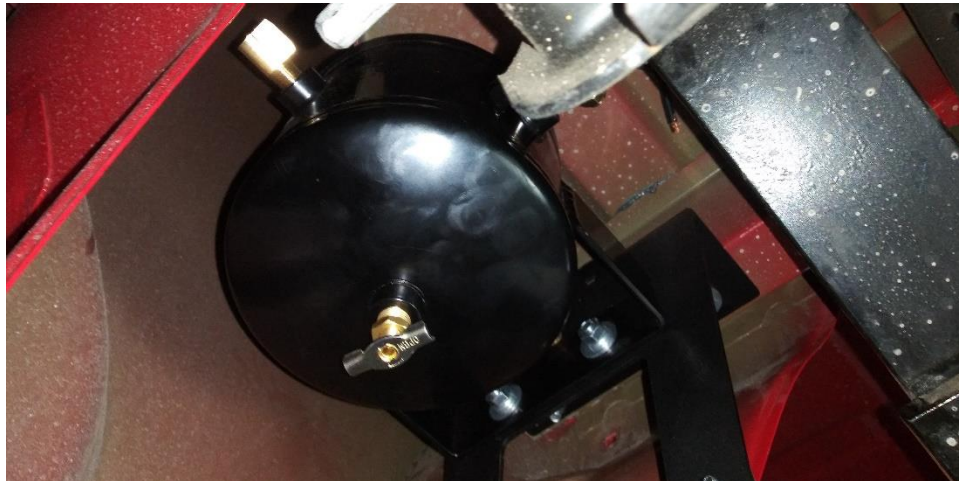
Figure 3 – Under Vehicle view of Air Tank Installed – Behind Driver Bed Side (2020 Silverado Shown)
