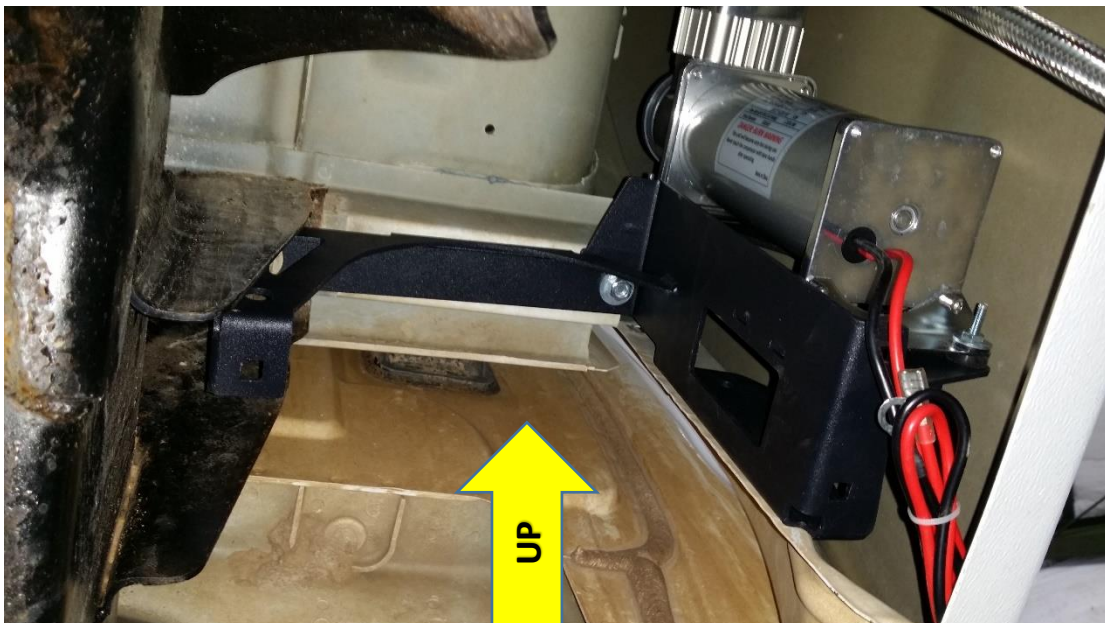
Figure 20 - Air Compressor Bracket Assembly, installed
