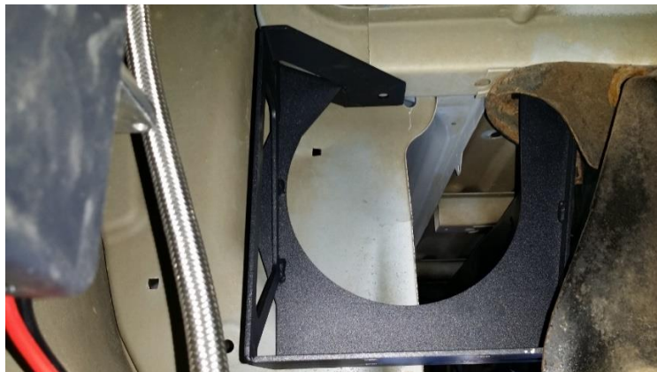
Figure 23 - HD18-201 Air Tank Bracket, installed
