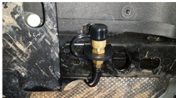
Figure 28 - Example of Air Coupler Mounted below Bumper
