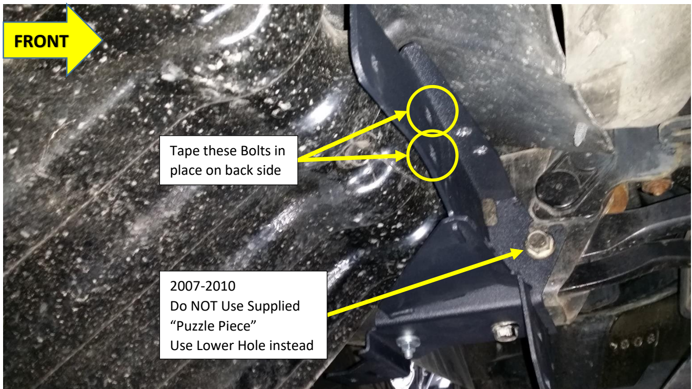
Figure 33 - (2007-2010 ONLY) HD18-301, Driver Side Bracket, installed without Puzzle Piece
