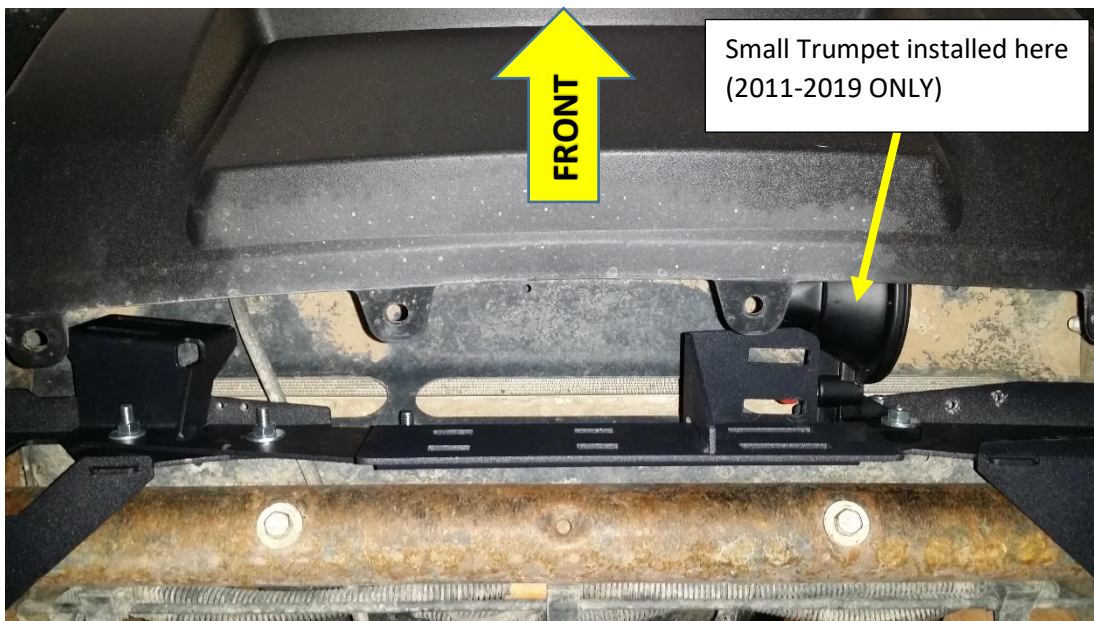
Figure 37 - HD18-303 Connector Bracket, installed (Shown from below)
