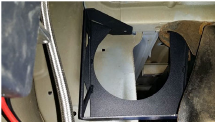
Figure 23 - HD18-201 Air Tank Bracket, installed
