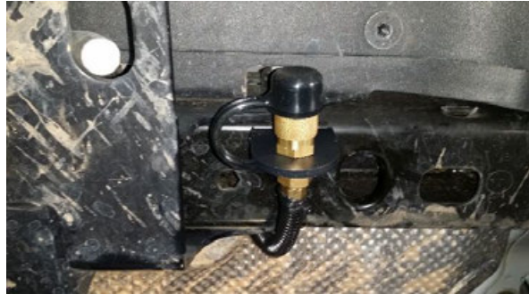
Figure 28 - Example of Air Coupler Mounted below Bumper
