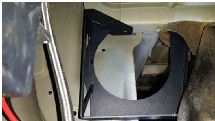
Figure 23 - HD18-201 Air Tank Bracket, installed
