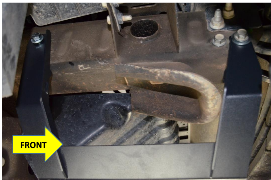
Figure 14 - Bracket Installation to Frame Rail (Passenger Side)
