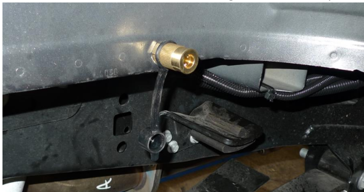
Figure 19 - Compressor to Air Tank Line
