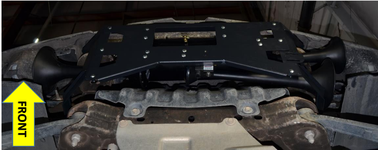
Figure 23 - Trumpets Installed before Wiring/Plumbing
