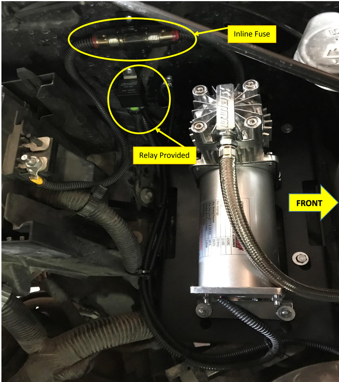
Figure 3 – Compressor Mounted, with Wiring Recommendation
