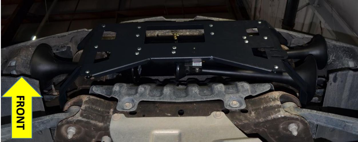
Figure 23 - Trumpets Installed before Wiring/Plumbing
