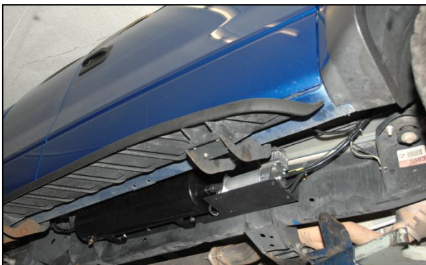
Location of Air System (Passenger Side)
