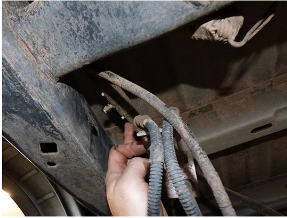
Image G – Separate wiring harness from frame
