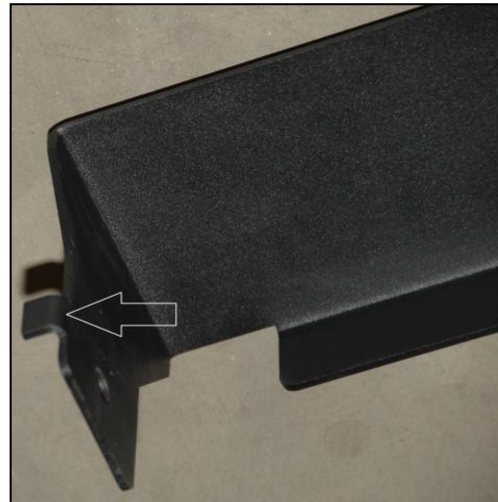
Image J– Horn Mounting Bracket stabilizing tab
