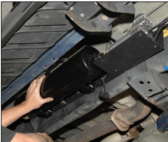
Image C - Air Tank Location on Frame
