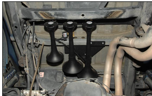
Location of Air Horns (Under Bed Floor – Model 730 shown)
