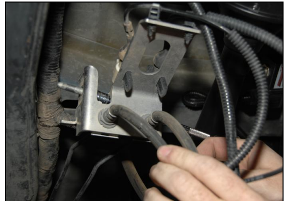
Image F – Brake Line Bracket
