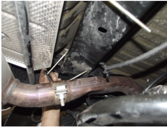
Photo 3 – Slide the rear mount plate/bolt assemblies over the beam. Work from the driver's side and slide the assemblies towards the passenger's side
