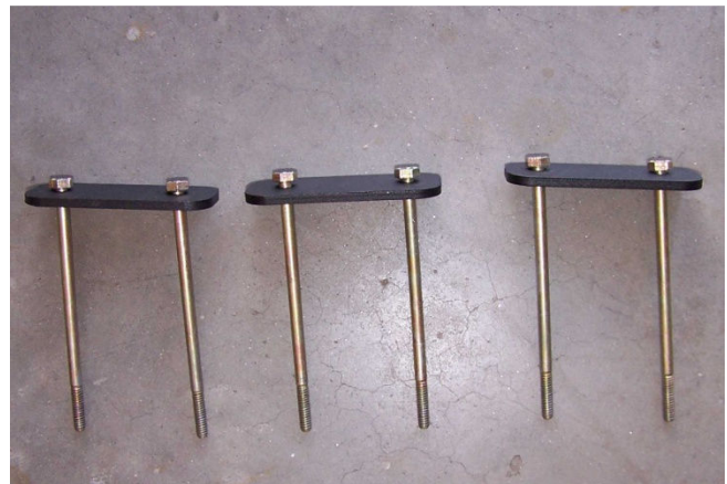
Photo 2 – Rear Mount Plates with bolts inserted
