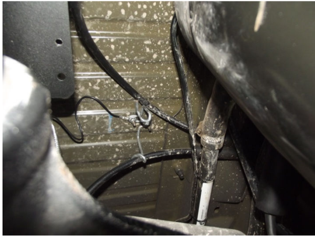
Photo 7 – Emergency brake cable support
