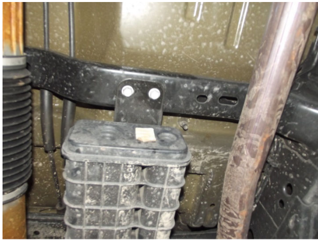
Photo 9 – EVAP canister. Note the two 5/8” mounting bolts
