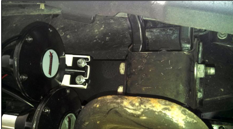
Figure 5: Horn Mount Installed with Tow Hook:
