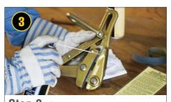
Step 3. Spray degreaser on the grip jaws, all joints and moving parts.
