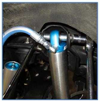
5. Install reservoir brackets – You will need to drill two holes in the pinch seam to mount reservoir. Measure back (7 inches) from the shock mount as shown. Measure up 5/16 and center punch. Drill 1/4" hole.
