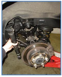
3. Slide the provided spacer onto the lower mounting stud as shown, then place the rod end on the stud. Install the provided bolt with washer and tighten to factory specs. Do not reuse the factory bolt.
