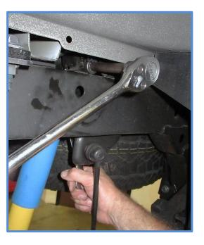
3. Install King Shocks by placing the end cap in the upper mount with the reservoirs facing away from the axle and the longer bearing spacer facing the frame. Install the factory hardware and tighten to factory specs.
