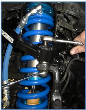
This kit does not require welding. Do not weld on any component. Welding may void the warranty and/or cause the product to fail.
