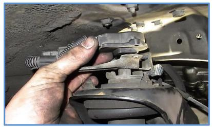
3. Remove bracket by holding nut on top of shock then remove the nut above the bracket.
