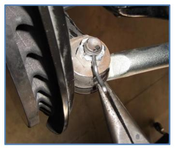
9. Remove lower mounting bolt using a 19mm wrench and socket.
