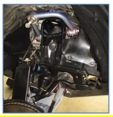
This kit does not require welding. Do not weld on any component. Welding may void the warranty and/or cause the product to fail.
