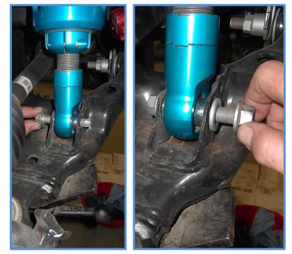
15. Jack up the lower control arm so the upper mounting plate is tight against the upper mount and install the 3/8 HD washers (CW1701) and 3/8 nuts (CN2711).
