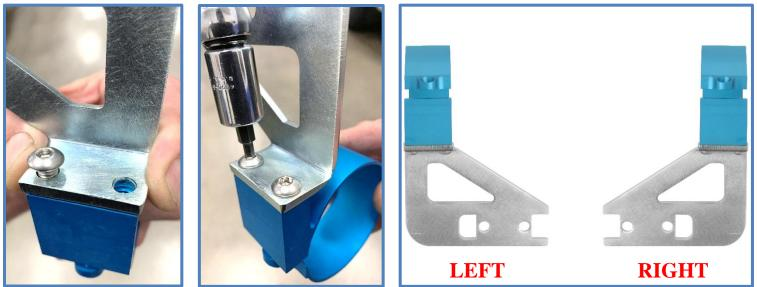
9. Insert the Backing Plate (25049-040) into the rectangular hole in frame with the rounded corners facing towards the front of vehicle. Flip the plate out with thumb as shown below and slide forward to hold in place.
