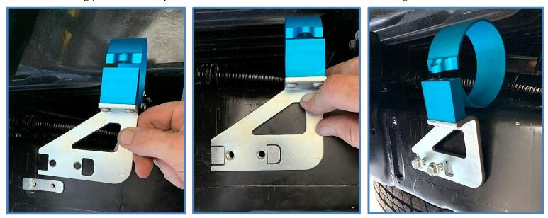
11. Slide the reservoir into the clamp as shown below.
