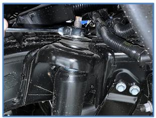
3. <u>Install Brake Line Bracket</u> – Remove the bolt holding the factory brake line bracket using a 12mm socket. Attach the provided Brake Line Bracket to the factory location using the factory bolt, then attach the factory brake lines bracket to the new bracket as shown below using the supplied 8mm bolt (CB3825) place the supplied washer and nut on the bolt and tighten.
