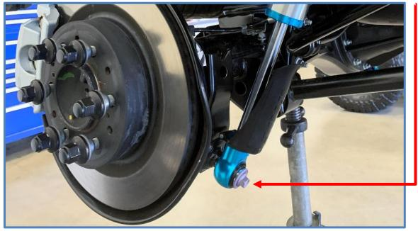
7. Tighten upper nut using a 3/4" wrench.
