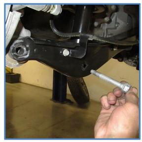
3. Remove the upper mounting nuts using an 18mm wrench/socket.
