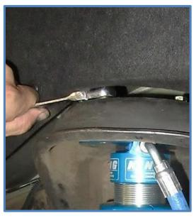
7. Install the lower mounting bolt and tighten to factory specs.
