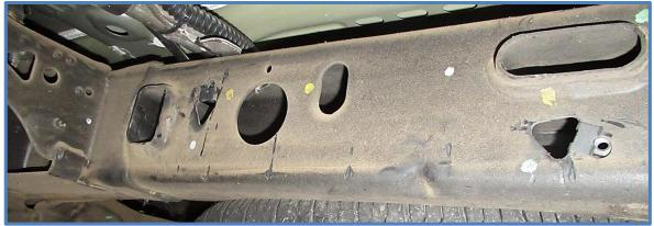
13. Attach reservoir bracket to the nut plates in the frame using the provided 1/4" bolts and washers...
