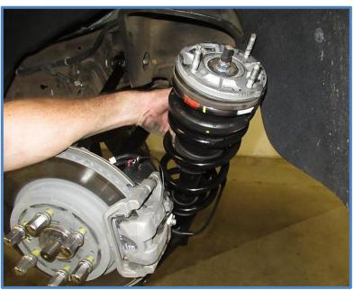
5. <u>Install King Shocks</u> – Be aware the shocks are side specific make sure you are installing shocks on the proper side. Place the shock in the lower mount, push down on lower arm and place the top of shock into the upper mount. You may need to jack the lower arm up to push the shock up into the upper mount so that you can get the bolts started in the upper mounting plate.
